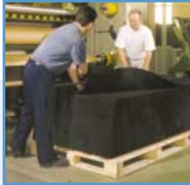
Two workers were employed stacking sheets of foam rubber on to pallets. The process required the sheets to be lifted at a rate of two to four per minute for an eight hour shift. Both workers had complained of muscular pains associated with performing this task, the taller complaining of low back pain from stooping, and the shorter of shoulder pain from repeated lifting above shoulder height.
